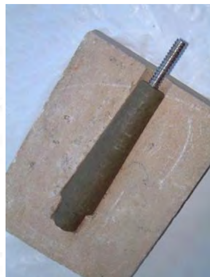
Fig. 5 Left, design detail showing the reverse tapered vertical reinforcing termination. Right, installed taper.
