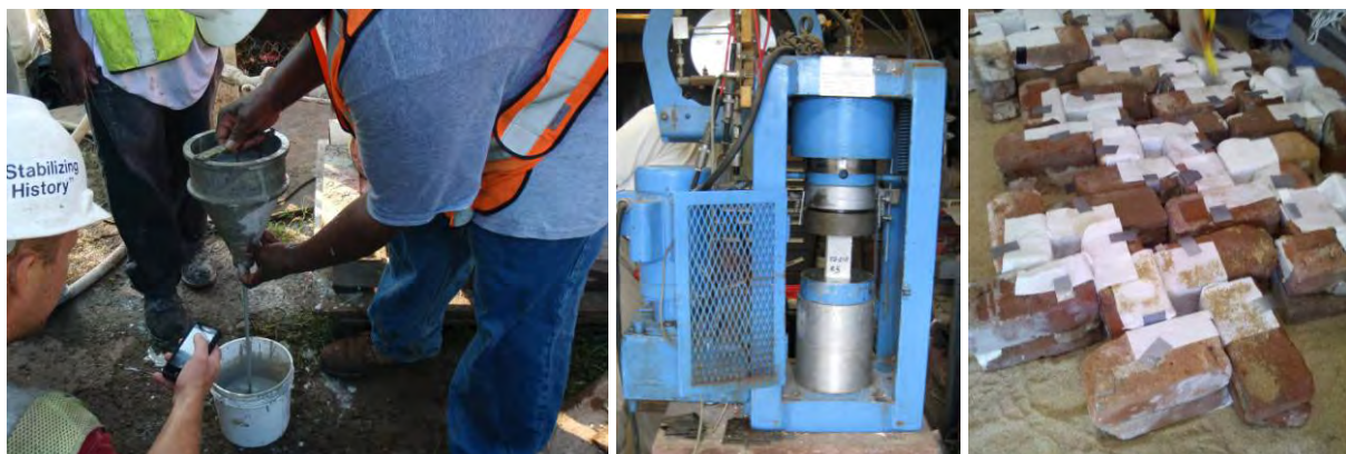
Fig. 8 Left, flow cone testing to verify viscosity of CIF material. Center, compression testing of a hardened CIF sample. Right, brick forms used to cast CIF compression samples.
