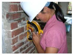
Fig. 1 Mortar rebound hardness, measured here using a pendulum hammer.
