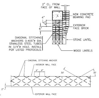
Fig. 4 Design detail showing diagonal stitching installed as confinement reinforcement: wall section (top) and horizontal plan section (bottom). Stainless steel tubes inserted into drilled holes were injected with CIF to bond new reinforcement to surrounding masonry.
