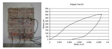
Fig. 3 Masonry deformability test conducted using the flatjack method. Test setup shown at left; at right is a typical stress-strain curve. Masonry compressive strength was measured to be in the range of 450 psi.
