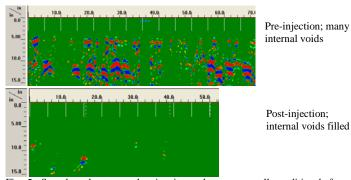
Fig. 5 Sample radar traces showing internal masonry wall condition before injection (top) with many internal voids as indicated by multiple reflections within the radar trace. Following injection the radar trace shows the wall to be essentially solid (bottom) with no significant reflections.
